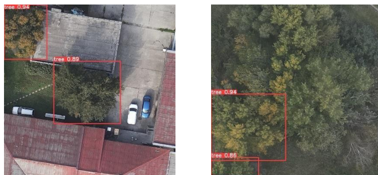
Figure 4. Tree segmentation in the orthophotomosaic using the YOLOv5 tool. The image illustrates the problem of detecting individual trees in the case of dense vegetation (continuous canopy).
